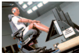
Dummy and seat on dynamic test sled.
